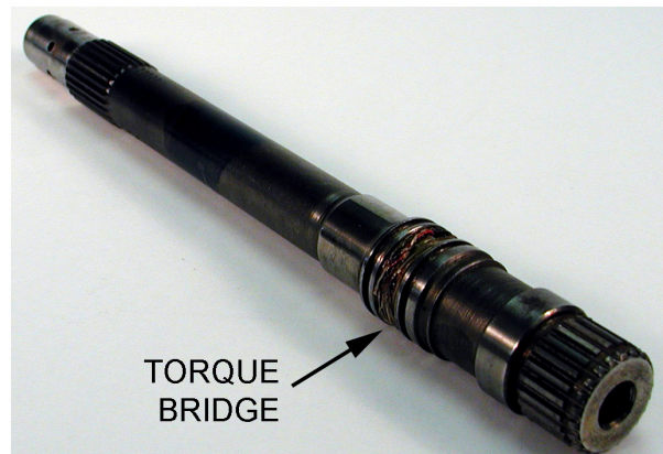
TRANSMISSION INPUT SHAFT - STRAIN GAGED AND CALIBRATED TO MEASURE TORQUE
