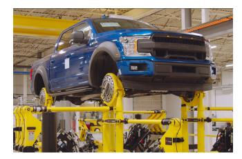
Forces recorded on test or durability tracks can be recreated on simulation rigs. Our instrumentation can be used for precise measurement on and off the track.
