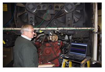
Experts can gauge components for strain and temperature on nearly any part of a vehicle. This data can confirm FEA and be used for vehicle development.
