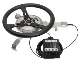
The *SW-SR2 Steering Wheel Torque and Angle Transducer* is capable of measuring the steering wheel torque, steering angle, and steering velocity on a full range of vehicles. *SW-SR2* has a ±1440 degree multi-turn encoder and both Analog and CAN signal outs.
