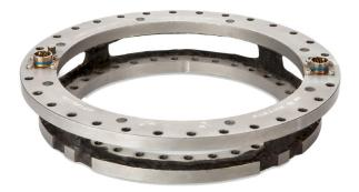
The *LW9.5 Wheel Force Transducer (WFT)* is capable of measuring all of the wheel forces and moments on ATVs, utility and other lightweight vehicles. It provides independent output signals for vertical, lateral, and longitudinal forces as well as camber, steer and torque moments. Completely weatherproof, it is ideal for off-road measurements in all weather conditions. It can also be used to monitor and control laboratory tests.
