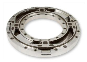
The *LW-MC-3.5K Wheel Force Transducer (WFT)* is capable of measuring all of the wheel forces and moments on a motorcycle. It provides independent output signals for vertical, lateral, and longitudinal forces as well as camber, steer, and torque moments. It is completely weatherproof making it ideal for testing in any weather conditions.
