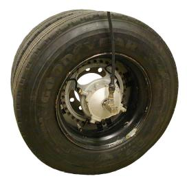
The *LW-1T-25K Wheel Force Transducer (WFT)* is capable of measuring all of the wheel forces and moments on a single wheel for class 8 trucks. It provides independent output signals for vertical, lateral, and longitudinal forces as well as camber, steer and torque moments. It is completely weatherproof making it ideal for on-road and off-road measurements. It can also be used to monitor and control laboratory tests. Two sensors are required for a dual wheel set, one for each tire.
