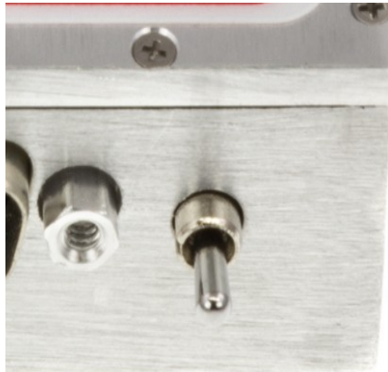
Figure 5: Switch selectable termination
