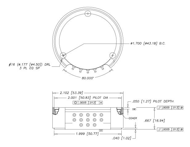
Three #8 socket head cap screws should be tightened to no more than 45 inch-pounds to secure the amplifier.
