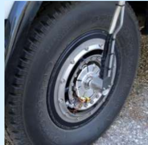
Complete assembly with slip ring, thermocouples, and spinning amp
