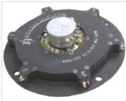
6-ch 1/4 arm strain gage spinning amp package
