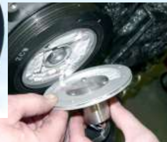
Strain gaged crankshaft with spinning amps
