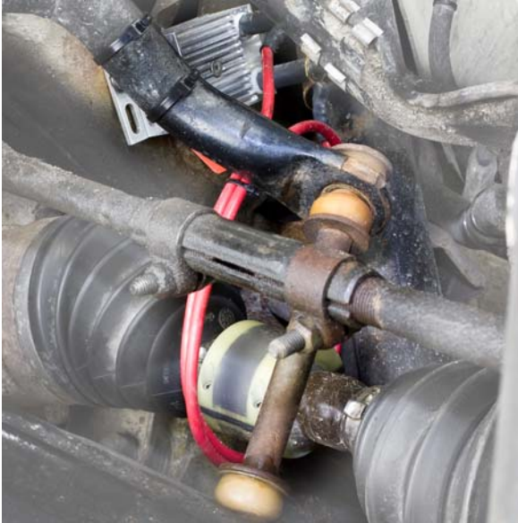
1.2" Split Collar installed on an automotive half shaft with a double loop induction primary coil.
