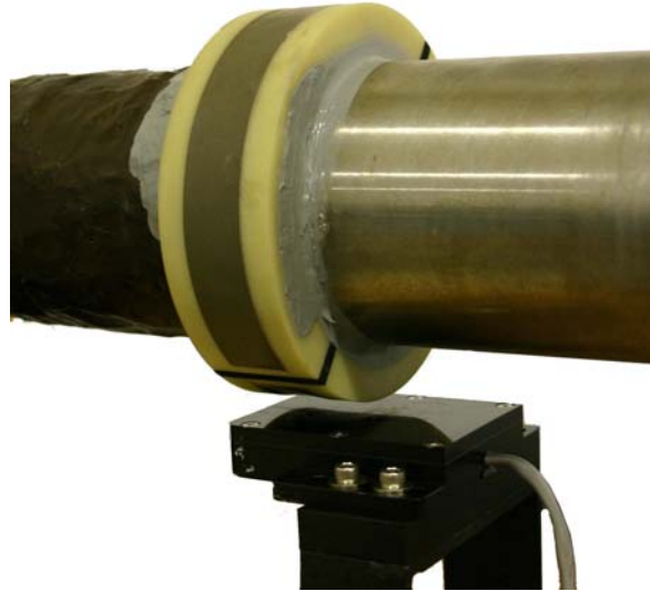
3.5" Split Collar Telemetry System installed on a wind turbine drive shaft with a "paddle" style induction primary coil.
